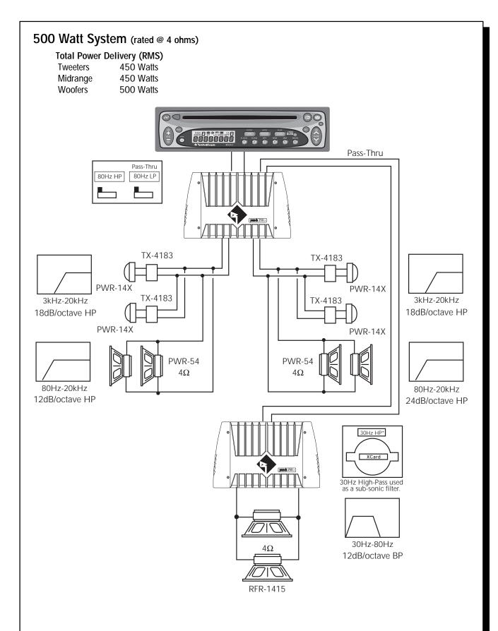
• A sub-sonic filter is a high-pass filter that limits the input signal below a certain motion below that frequency. At very low frequencies a woofer has no output, just motion. If you try to drive this woofer at these lower frequencies, the woofer could self-destruct. Please refer to the crossover section of the manual or see your local Authorized Rockford Fosgate Dealer for more information.
